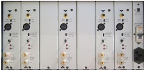
The five-way speaker binding posts are plastic, but sturdy. On the right are the grounded AC receptacle and a toggle circuit breaker. So, you don't need to replace fuses. When powered on, small LEDs on the front panel illuminate.
