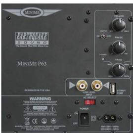
The MiniMe P63 amplifier utilizes the advanced class “D” circuitry with over 90% efficiency, allowing it to continuously perform without getting hot.
