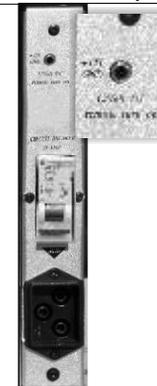
If you plan to power the Cinénova using an external source. Then you will need to plug the source into the 12VDC Trigger.
