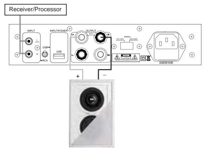
Wiring with the Q10B Tactile Transducer
