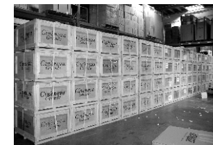
Wood crates are used to package these 150+lbs amplifiers to prevent any damages during shipping.
