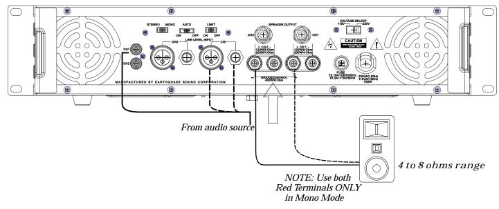
The following diagrams are excerpts from the system block diagrams and are intended to provide a simplified view of the operating modes of the amplifier.
