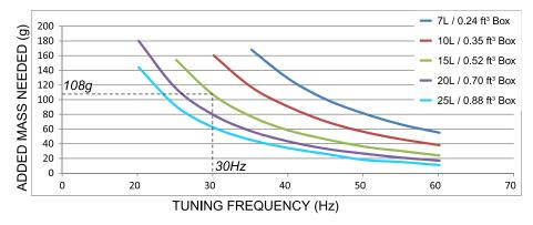
For example, the net internal volume of your speaker box is 0.52 ft<sup>3</sup> (15L) and your preferred tuning frequency is 30Hz. You will need to add about 108g of mass to the SLAPS-M8.
